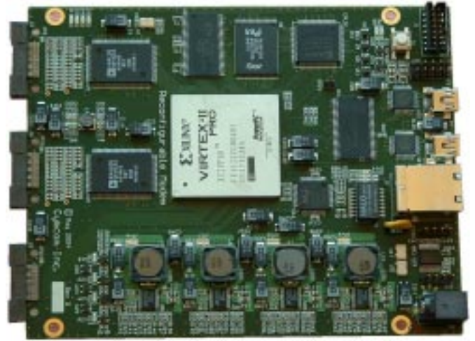
Xilinx Virtex-II Pro RF Development Board
